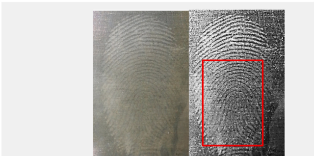
Fig. 10. [A] Photograph and high contrast image of latent finger-mark on a brass surface visualised in 2 mM EDOT and 1 mM thionine acetate in 0.1 M \text{NaNO}_3 at E_{app} = 0.1 V vs. \text{Ag}|\text{AgCl} for t = 120 s [B]: Photograph of and zoomed in high contrast image of visualised 5-month-old groomed latent finger-mark at E_{app} = 0.1 V vs. \text{Ag}|\text{AgCl} for 120 s split across two brass sheets showing left \text{NaNO}_3 and right EDOT-Th. Natural 16-month-old latent finger-marks on a brass surface visualised with EDOT-Th upon E_{app} = 0.1 V vs. \text{Ag}|\text{AgCl} for 120 s with [C] male and [D] female. [E] Average level of visualisation score for 16-month-old finger-marks showing both male and female donors for natural and groomed finger-marks.
