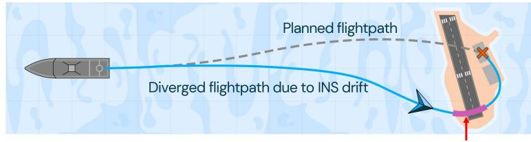
1. **Tactera Marine** gives enhanced INS linear drift over open-ocean of about 6km in 1 hour on a baseline \$5 IMU and getting better. 1km drift in 10 mins.
