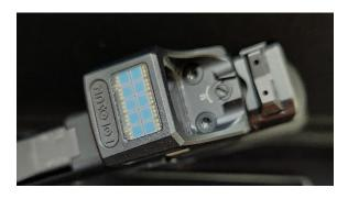
The top of the SCS Carry features a multidirectional solar charging panel. This panel is designed to capture ambient light from various angles, maximizing its efficiency in converting light into electrical energy. This solar energy directly powers the optic in sufficient lighting conditions, significantly reducing the drain on the internal battery. It works with both natural sunlight and artificial light sources. Even indoor lighting can contribute to powering or charging the internal battery.
