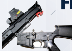
AR-type MCD on lug of upper assembly
