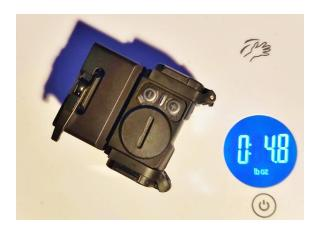
With a battery installed and mounted on the B&T mount, the ACRO C-2 weighs only 4.8 ounces. The sight and mount package measures 2.29 inches overall and two inches to the center of the aperture, and seamlessly integrates with most setups without requiring adjustments to stock height or cheek weld.
