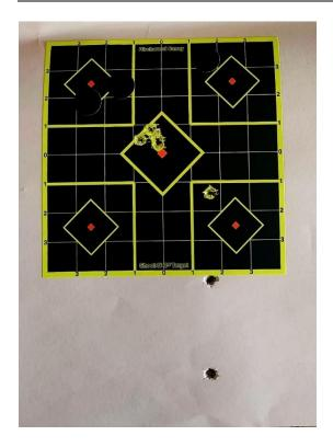
The key takeaway from the image above is not the impressive 3-shot group at 25 yards. My focus is on the precise vertical movement of the point of impact as I zeroed the sight. This demonstrates the lack of wind influence on elevation adjustments.
