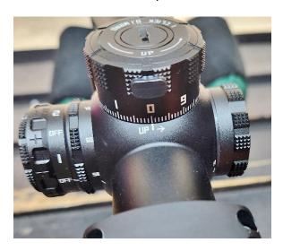
Once zeroed you can reset your turrets to "0" by removing the turret dial and aligning the "0" mark with the indexing mark provided.
