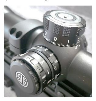
and parallax. The outer dial handles illumination, which is activated by pulling out and rotating the dial to the desired brightness level. To secure the setting, simply push the dial back in. Six illumination levels are available, separated by off positions. The TANGO DMR's locking illumination system is a standout feature. It prevents accidental changes to brightness settings, ensuring consistent reticle visibility.
